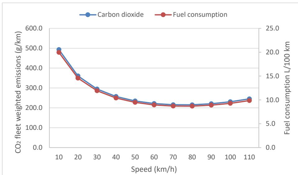
**Figure 1: CO<sub>2</sub> and fuel consumption fleet weighted emission factor versus speed (2018)**
