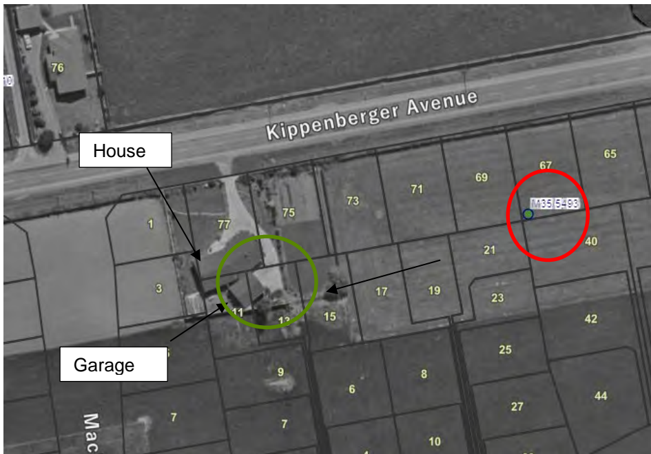
Figure 6 Approximate location of M35/5493 (green circle) based on sketch map from wells database and 1970-1974 historical aerial photograph (Canterbury Maps), compared to mapped location (circled in red)
